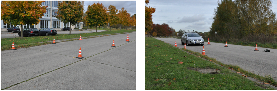
Figure 1.2: Arrangement of the traffic cones serving as a reference in the scan data.
