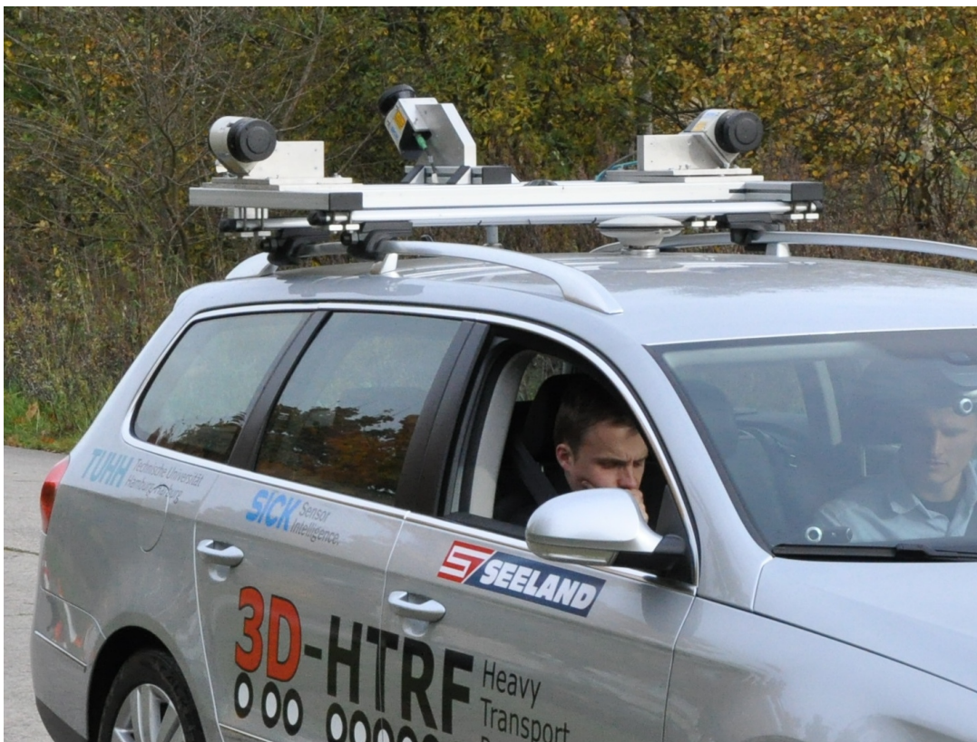
Figure 2.2: The Volkswagen Passat used by Gustav Seeland GmbH with three SICK LMS151 laser range finders on the roof. One LRF to scan each side of the car and a third on the stern of the car.
