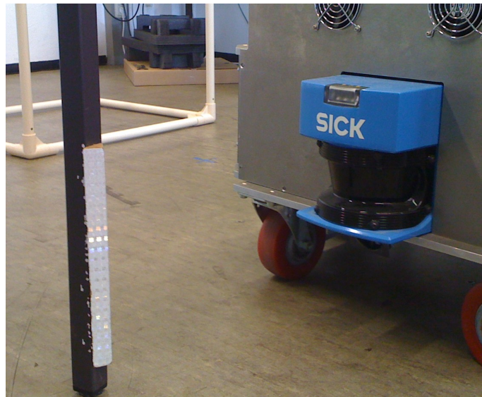
Figure 4.6: A SICK laser scanner and a reflector-mark installed on a table leg for an easily recognition
